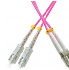
Patchcord SC/UPC-LC/UPC, MM, 50/125 duplex, OM4 fiber, 5 m
