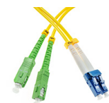
Patchcord SC/APC-LC/UPC, SM, 9/125 duplex, G652D fiber, 5 m
