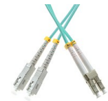
Patchcord SC/UPC-LC/UPC, MM, 50/125 duplex, OM3 fiber, 2 m
