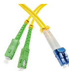
Patchcord SC/APC-LC/UPC, SM, 9/125 duplex, G652D fiber, 2 m
