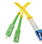
Patchcord SC/APC-LC/UPC, SM, 9/125 duplex, G652D fiber, 3 m
