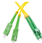
Patchcord SC/APC-LC/APC, SM, 9/125 duplex, G652D fiber, 10 m
