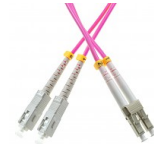
Patchcord SC/UPC-LC/UPC, MM, 50/125 duplex, OM4 fiber, 1 m
