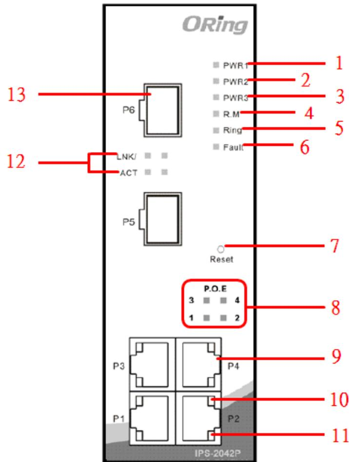
1. LED for PWR1. When the PWR1 links, the green led will be light on.
