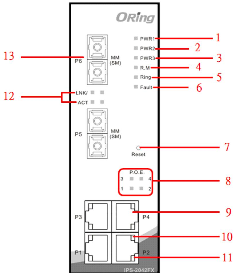
1. LED for PWR1. When the PWR1 links, the green led will be light on.
