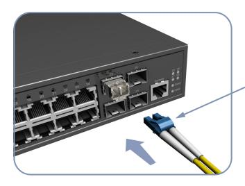
For fiber transceivers connect 62.5/ 125 or 50/125 multimode or 9/125 single-mode fiber with LC connectors.
