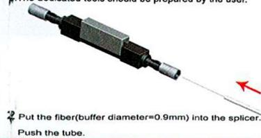
2 Put the fiber (buffer diameter=0.9mm) into the splicer. Push the tube.
