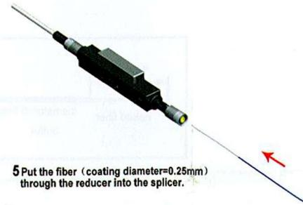
5 Put the fiber (coating diameter=0.25mm) through the reducer into the splicer.
