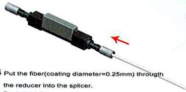
4 Put the fiber (coating diameter=0.25mm) through the reducer into the splicer. Push the tube.
