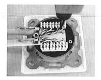
Place the cable(s) underneath the M-shape cable holder properly, make sure the foil or braid shield contact with the cable holder, and then fasten the screw.
