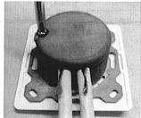
Adjust the gap on the cover to fit the cables. Latch the snag (the circle in the figure above) to the hole on the body and then fasten the screw.
