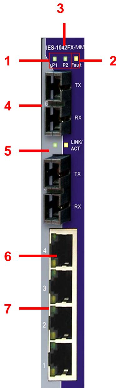
1. LED for PWR1&PWR2. When the PWR links, the green led will be light on.
