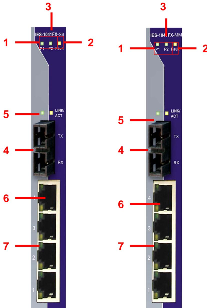
1. LED for PWR1&PWR2. When the PWR links, the green led will be light on.
