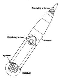
4.17 Network cable integrity test
