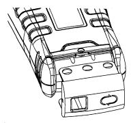
4.19.3 The figure below shows how the protective cover is used when the cable detection function is not used.
